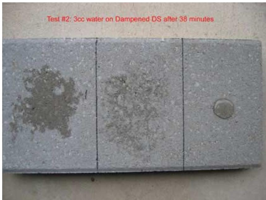
After just under an hour, the 3 ccs of water has almost completely dried where it was applied on top of the Deep Seal....while the 3 ccs applied on the left untreated section still shows dark indicated presence of water.
