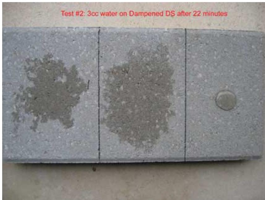
By 25 minutes the difference in drying between the left and middle sections is becoming more evident... with the DS treated area getting dry faster than the untreated section on the left, which is darker in color, indicating more moisture present.
